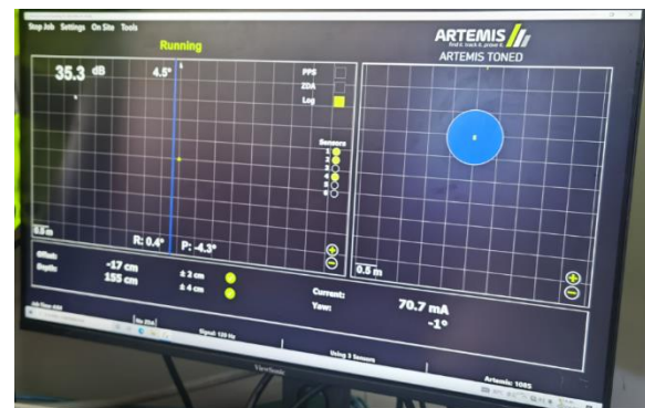
Figure 11 - Operator display showing plan view (X-Y) and front view (Z) position of cable
