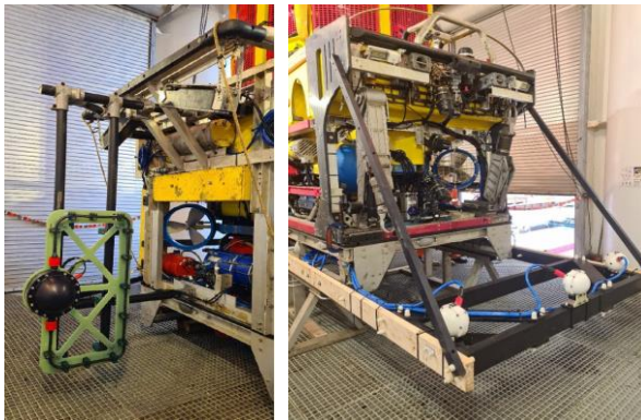
Figure 7 – Antenna and 3-Sensor Array on FCV3000 Survey ROV
