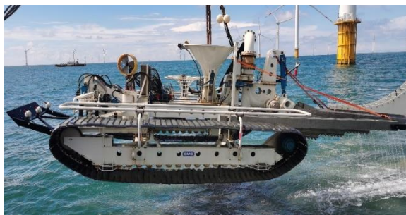
Figure 10 - Trencher with forward sensor array and (obscured) rear array
