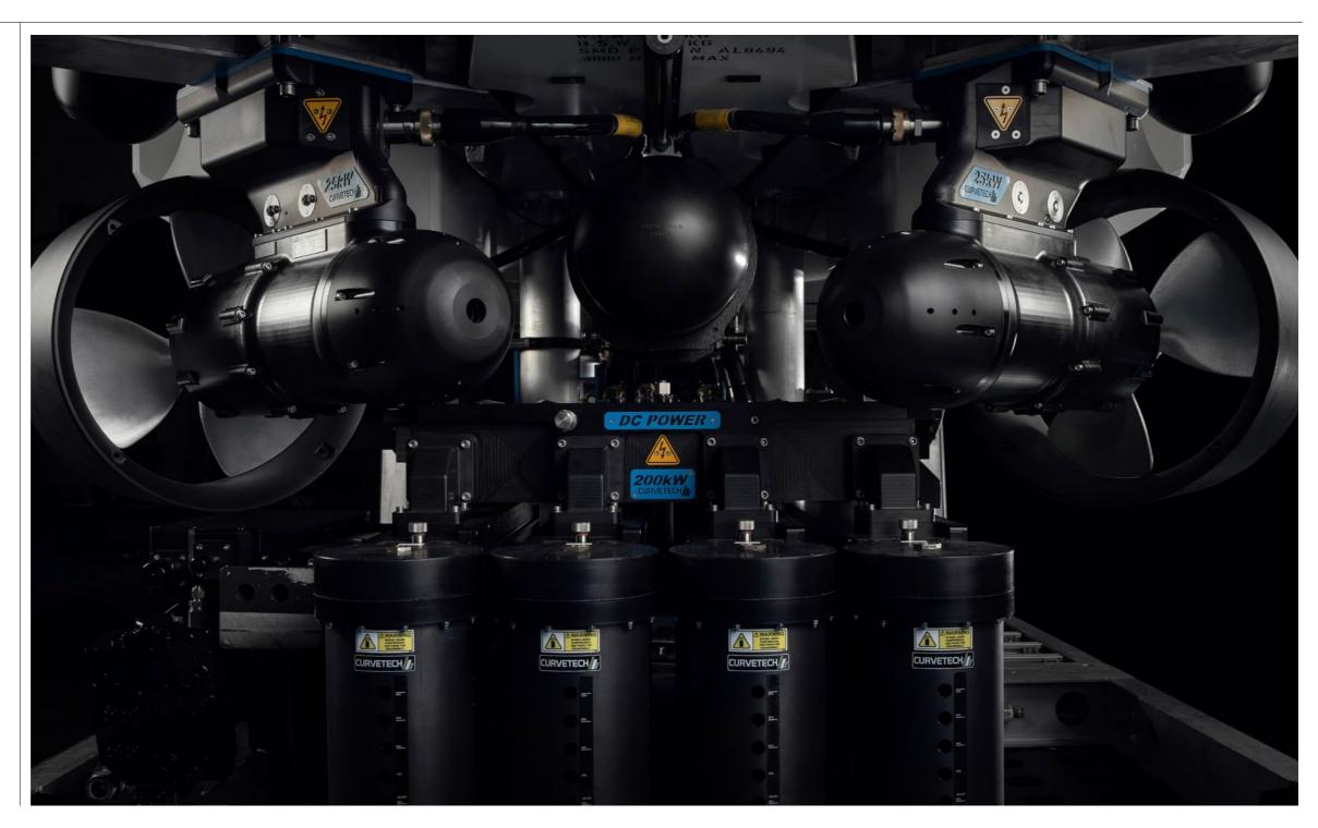
VEHICLE SPECIFICATION GENERAL Depth rating 3000msw Standard Optional 4000, 6000msw Dimensions Length ≤3306mm ≤1800mm Width ≤1900mm Height Weight in air (full construction spec) 4050kg Payload 400kg 4000kg Through frame lift Aft TDU mounting TBC PERFORMANCE Bollard pull (actual) Forward/aft 1300kgf 1300kgf Lateral Vertical (up) 1500kgf Surface performance Forward 4.5kn 3.5kn Lateral Vertical 3.7kn Auto functions Heading Depth Altitude
